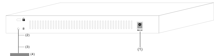
Figure 2-4 Install with grounding bar
